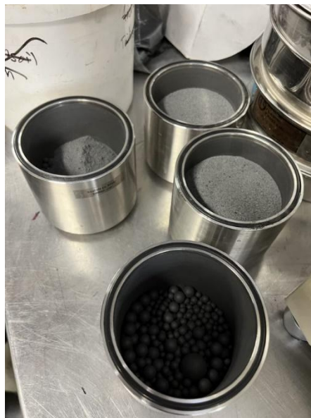
Fig. 3.4: Ball Milling Jars containing Steel Balls and FBA.
