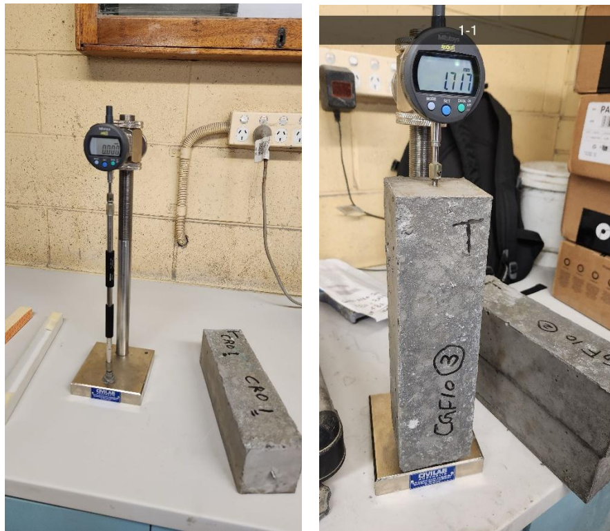
Fig 5.3. Shrinkage test setup.
