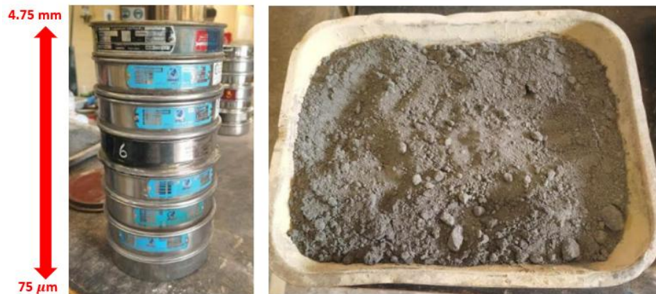
Fig. 3.1: Sieves (left) and raw FBA which has been oven dried (right).
