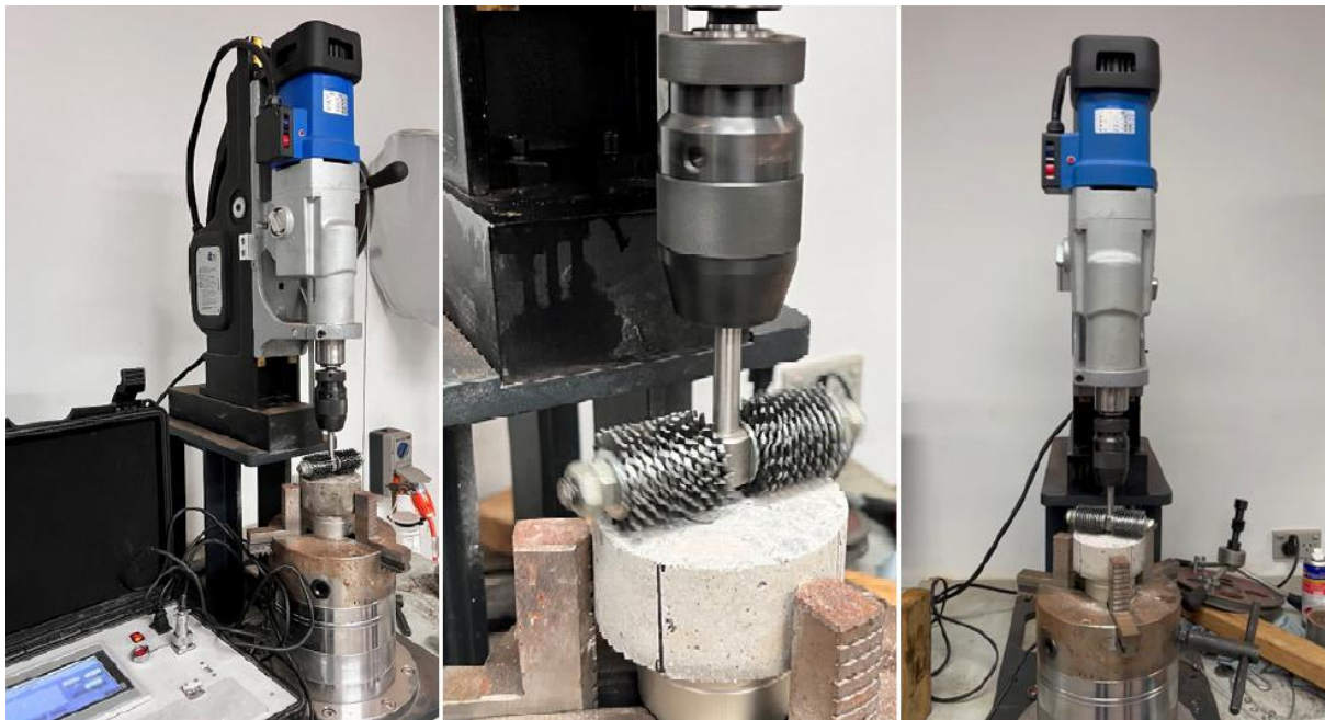
Fig. 5.13: Apparatus of Abrasion Resistance Test.
