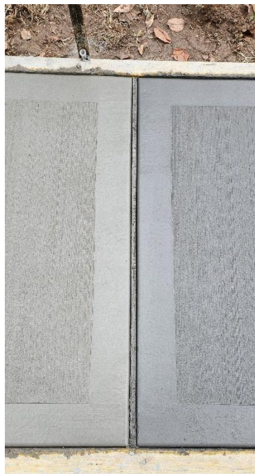
Fig. 6.10: Colour differences of Two mixes (FBA darker).
