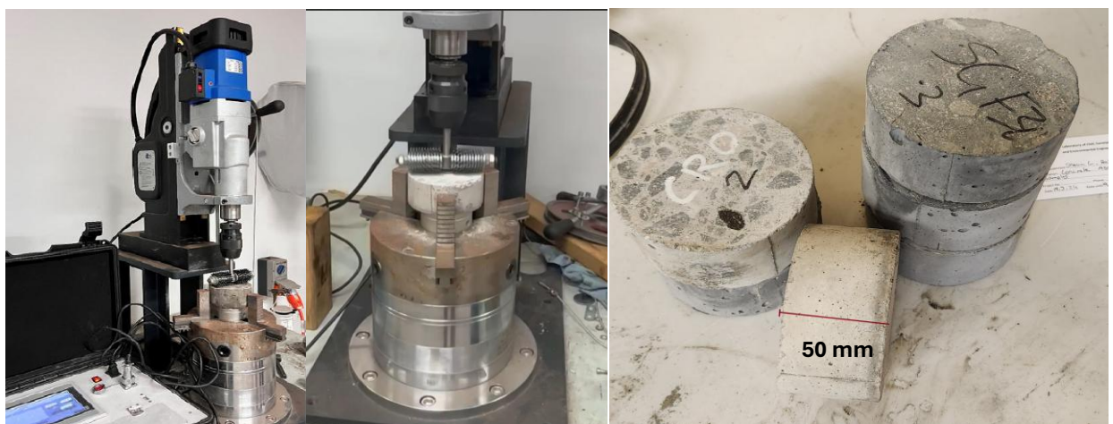
Fig. 5.1: Apparatus, test samples and setup of Abrasion Resistance Test.
