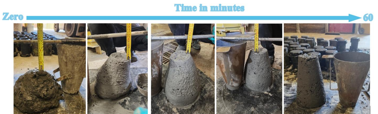
Fig. 5.5: The workability performance of designed concrete; a) initial slump and slump retention results, and b) actual photo of UON lab for CGF10 slump retention.
