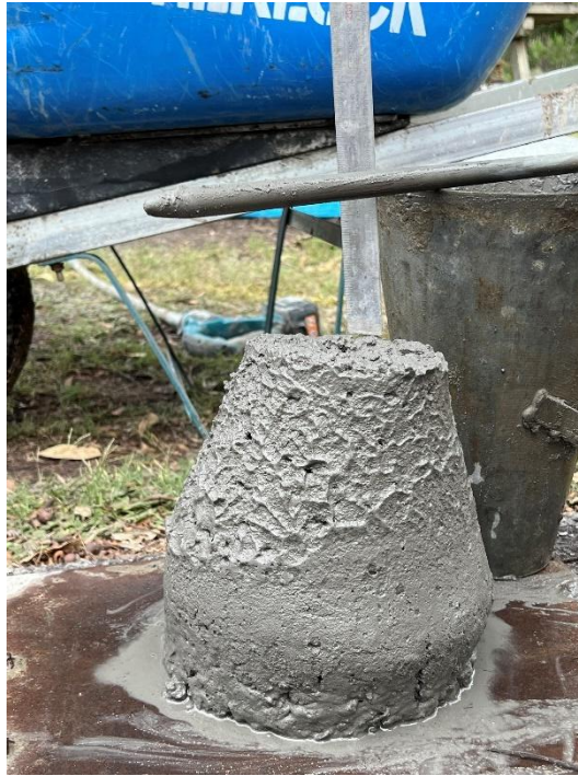
Fig. 6.9: Slump of FBA Concrete Mix.
