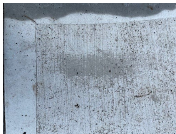
Figure 15: Dusting on FBA concrete (after two months)
